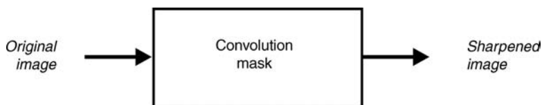
FIGURE 10.18 Unsharp masking process using convolution mask.
