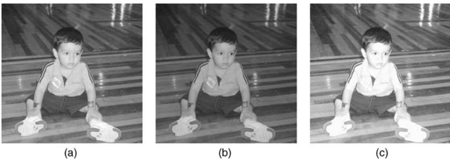
FIGURE 6.6 Multiplication and division by a constant: (a) original image ( X ); (b) multiplication result ( X \times 0.7 ); (c) division result ( X/0.7 ).
