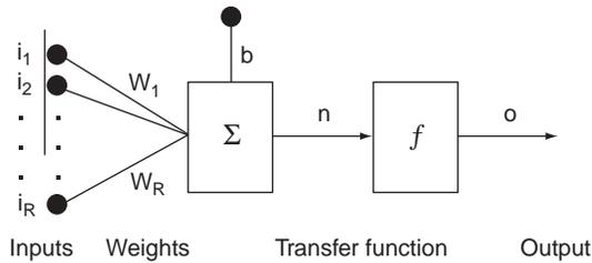
FIGURE 28.1 The concept of a neural network.
