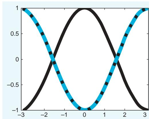
**FIGURE 23.1** Testing the second derivative function `secDer.m`. The solid black line is the input,  $\cos(x)$ , and the blue line is the output of the `secDer` function with periodic boundary conditions. This matches exactly with the analytic solution to the second derivative,  $-\cos(x)$ , shown as the dotted black line.
