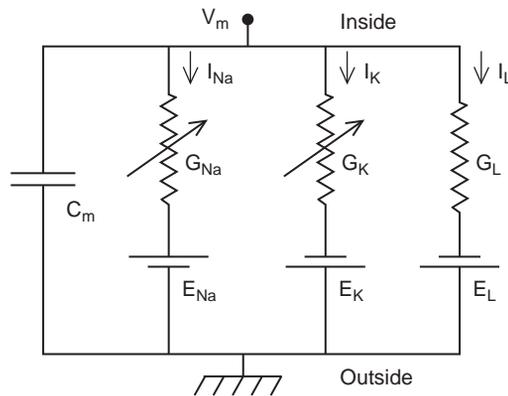
**FIGURE 20.2** An electrical circuit diagram of a single axonal compartment of a neuron. (Bower JM, Beeman D. *The Book of Genesis: Exploring Realistic Neural Models with the GEneral NEural Simulation System*, 2003)
