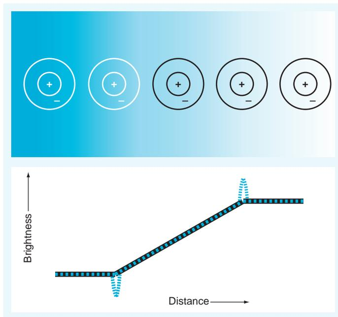
**FIGURE 10.1** The Mach band illusion. Top of figure: the visual stimulus with various center-surround receptive fields superimposed. Bottom of figure: the actual brightness of the visual stimulus (black solid line) and the perceived brightness of the optical illusion (blue dotted line).
