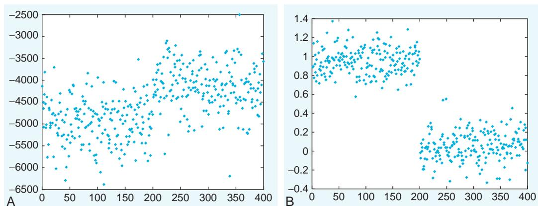
**FIGURE 29.6** The problem of categorizing “good” from “bad” Greebles using a supervised linear network. A. Classification when all the weights are set to 1 (Before training). B. Classification after application of the supervised learning rule (After training).
