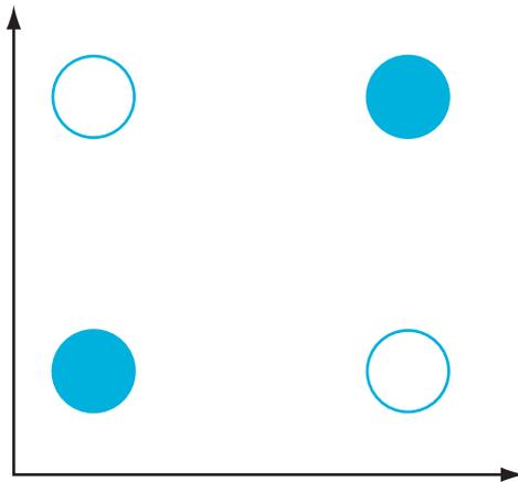
**FIGURE 29.1** The XOR problem that a single layer network cannot solve. The XOR problem requires that the neuron respond (i.e., white circles) when only one of the inputs is on but not both. This is not solvable by a single-layer perceptron or linear network because it is not linearly separable.
