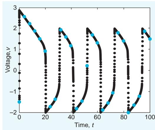
**FIGURE 23.2** Voltage,  $v$ , versus time,  $t$ , output of Fitzhugh-Nagumo system of equations for one point in space found using the `ode45` solver with `tspan=[1 100]` (black dots) and with `tspan=[1:4:100]` (blue dots.)
