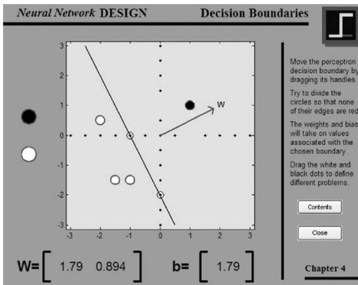
**FIGURE 29.2** An interactive display of the decision boundary of a perceptron provided in Neural Network Toolbox in MATLAB. The display shows how a perceptron creates a linear decision boundary whose slope and intercept can be modified by adjusting the weight vector and bias.
