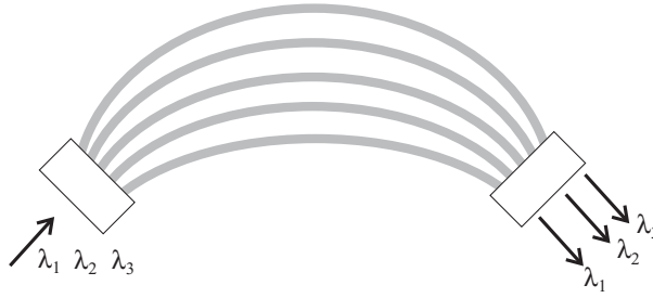
Fig. 13.3 Schematic illustration of a simple array waveguide demultiplexer.
